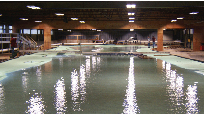
This model of the Smithland Locks & Dam will be used to test the effect that building a hydroelectric plant at the real locks & dam will have on river conditions and shipping.
